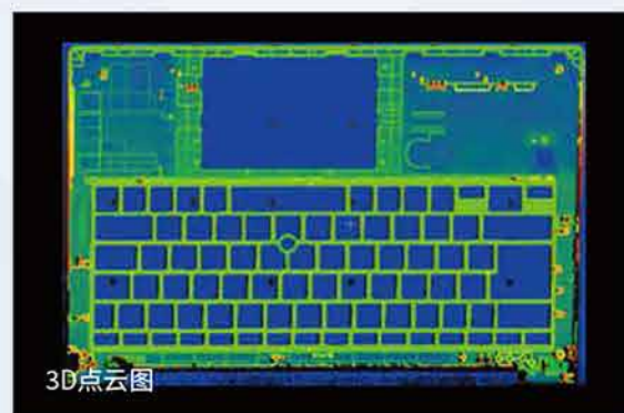
笔记本外壳检测 LAPTOP SHELL INSPECTION
